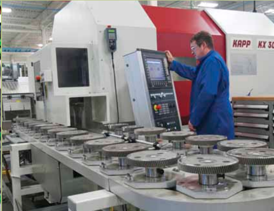
Gear grinding capable up to 300 mm, module 5, AGMA 14
