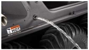
Bilge Pump A built-in bilge pump quickly and effectively evacuates water that enters an ARGO XTV.
