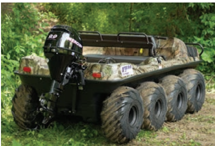
For greater speed on water add an outboard bracket and up to 9.9 hp motor.
