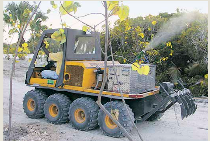
ARGO 8x8 Centaur with Arro-Gun sand fly abatement spraying system.
